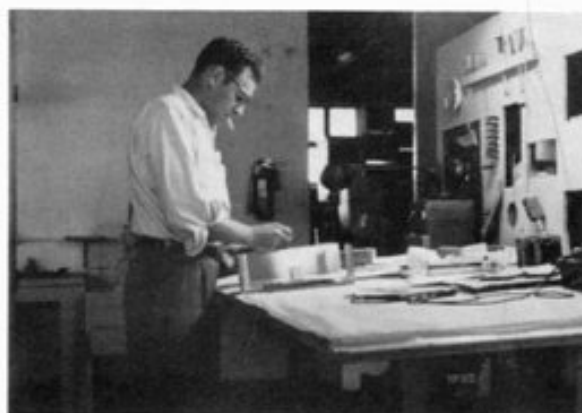
■ Bob Carver is shown here wiring a remote control unit in the company's downtown factory. This piece of equipment is slated for the famous Coast Guard Cutter, Mackinaw.
